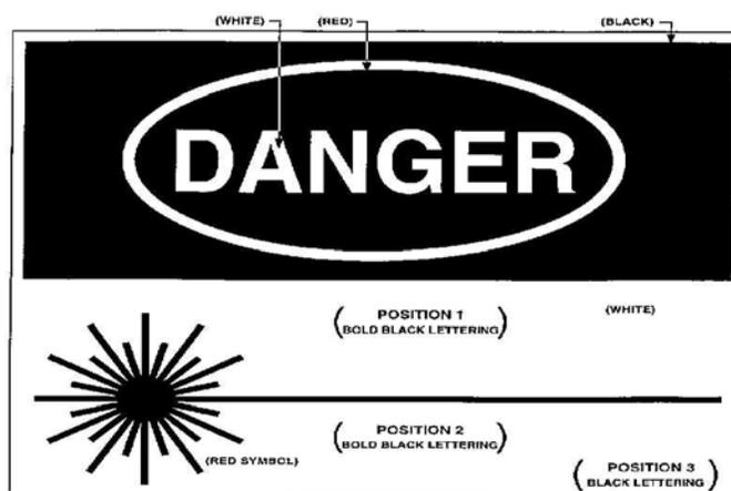
Figure 4. Area Posting for Class 3b and 4 Lasers
