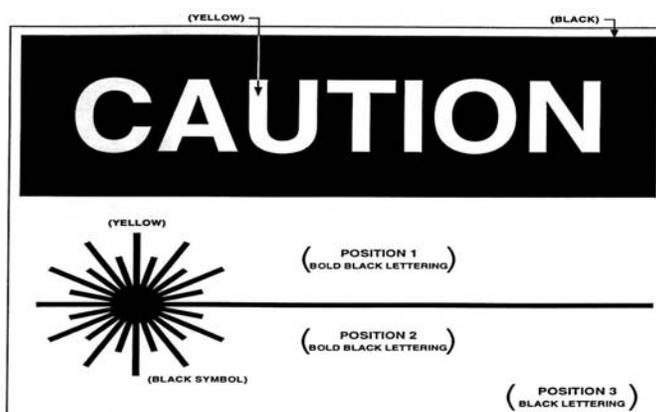
Figure 3. Area Posting for Class 2 and 3a Lasers
